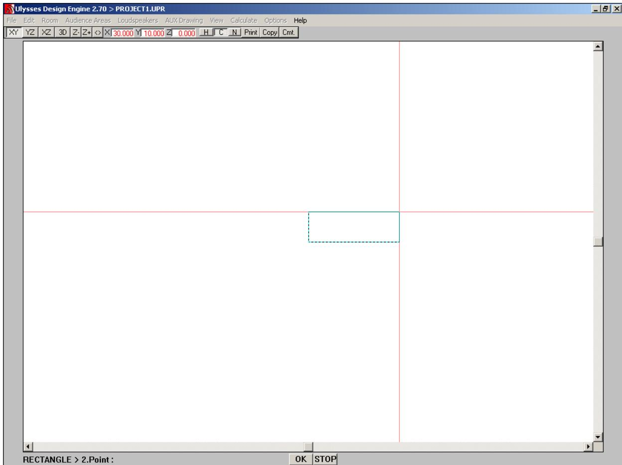
The second rectangle point has now been determined and the rectangle has been drawn. The Input Requirement line disappears.
