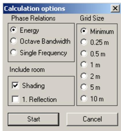
Select »Energy« from the »Signal Coherence« section (this calculates the energetic total of all sources, without interference effects). Do not select any of the »Include Room« options (i.e. no »checks«).
