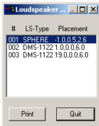
A speaker **highlighted blue** on the list is shown **red** in your model. Step thru loudspeakers via the cursor keys or by clicking on a loudspeaker of interest.
