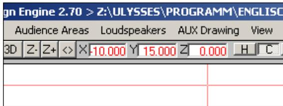
Because we want to draw the floor, **z** should read **zero!** If the z coordinate does not read zero, change to the yz view. Move the cross-hairs cursor until  $z = 0$  and change to xy view by striking F1.
