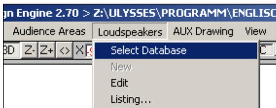
Without loading a speaker database you will be asked to do so when clicking on one of the Change Speaker buttons. In this case return to the main menu by closing the loudspeaker list.
