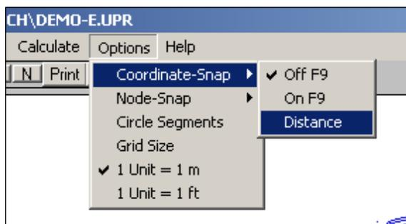
In the **»Options«** menu also click on **»Coordinate-Snap«** and **»Distance«**. Set **distance** to **5** in the input box. This will cause the cursor to snap at every 5 m or 5 ft. increment.
