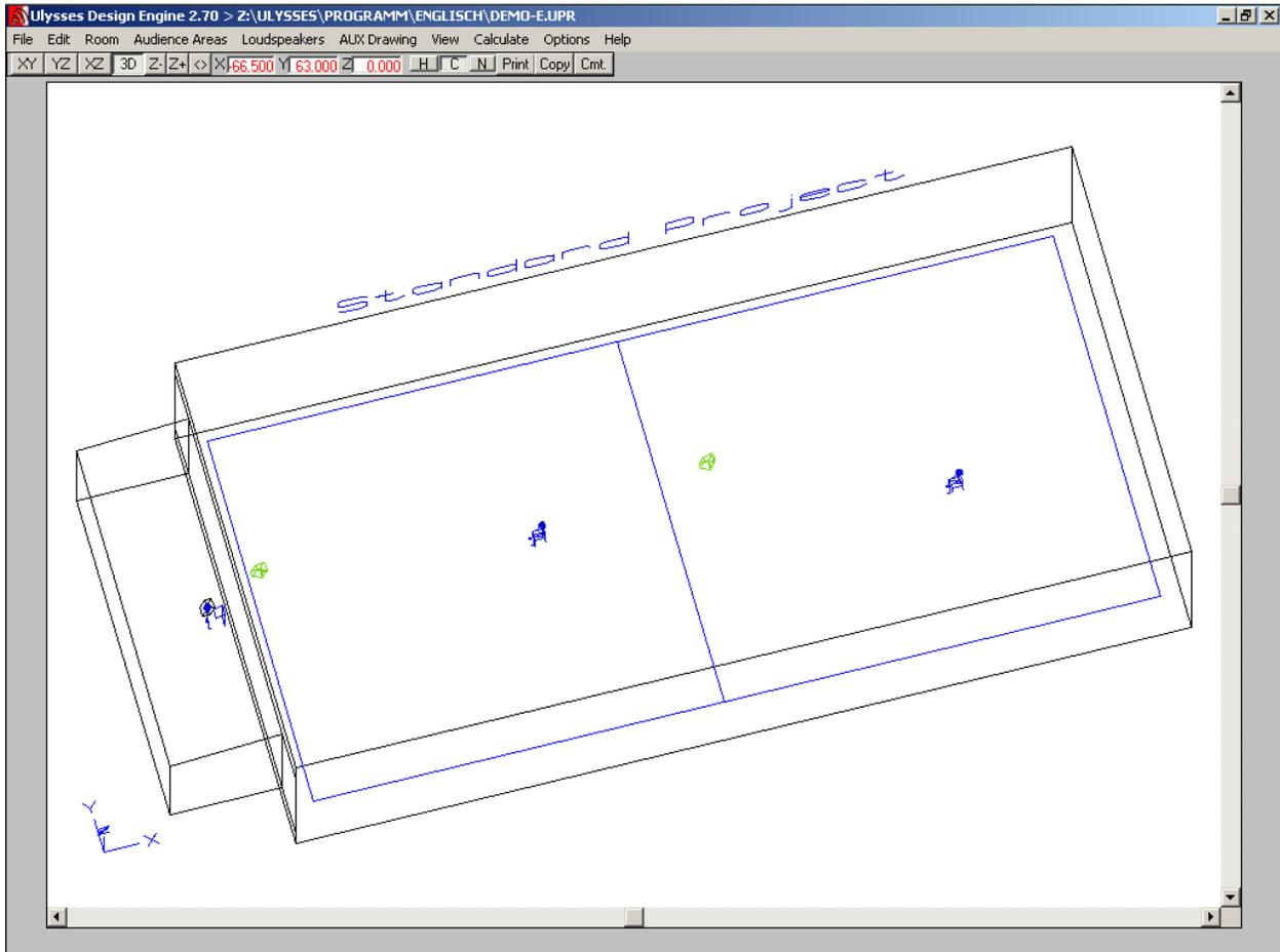
Clicking on the **XY** **YZ** **XZ** or **3D** in the top menu bar (or striking F1 - F4) toggles between model views.
