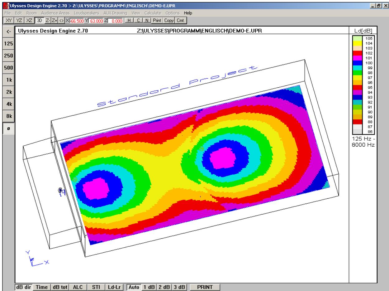
After calculation click on the different **frequency band buttons** left of the screen.
