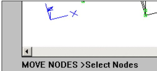
Select the **4 nodes** of the rear wall of the room. You may select other nodes by repeating above procedure. The selection of Nodes is terminated by RightClick or striking the Return or Space keys.
